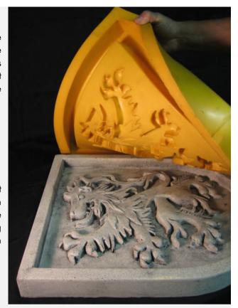
These elastomers are typically used in concrete molds, architectural shapers, filtration units and many more. With their flexibility, durability and various application advantages, elastomers play an important role in industrial and architectural fields.
